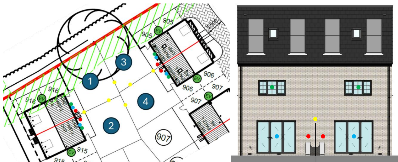
Figure 6: Layout of microphone positions with respect to the 4 properties. Fence microphones in yellow, ASHP microphones in red, patio door microphones in blue, and bedroom window microphones in green. Left: Plan view. Right: Elevation
